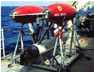
Figure 7: The Autonomous Benthic Explorer is an AUV that has created some of the most detailed maps of the seafloor terrain (“History of Oceanography”).
