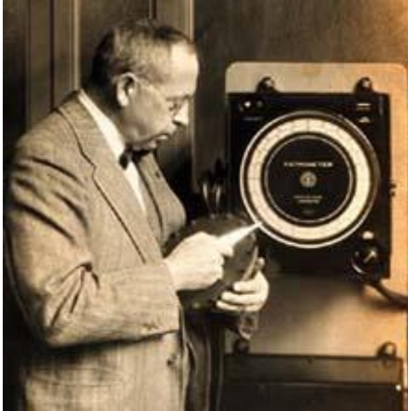
Figure 4: Herbert Dorsey with the Dorsey Fathometer around 1930 (NOAA Photo Library) (“Age of Electronics (1923-1945)”).
